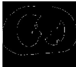
Fig. 4: Output image after sobel edge detection
